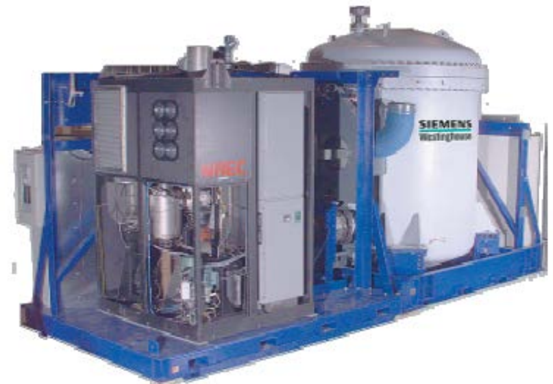
Fig. 7. Pressurized 220 kW SOFC/Gas Turbine Hybrid
